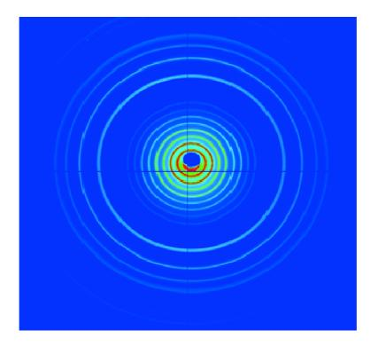
**Figure 1. BL11-NCD**: A 1 second exposure of silver behenate collected on an ADSC210 CCD detector with a sample to detector distance of ca. 220 mm is illustrated.
