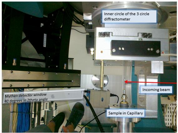
**Figure 2. BL04-MSPD.** SRM 640b - Silicon X-Ray Diffraction (from NIST) loaded on 1 mm diameter capillary is shown from the top of the experimental set-up.
